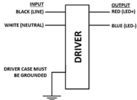
Input and output use lead- wires.
