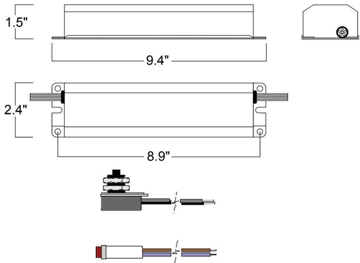
A test switch and charging indicator light are provided.
