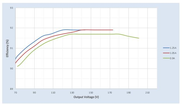
Efficiency Vs. Output Voltage at 277Vac
