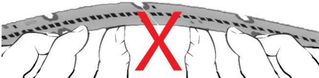
Figure 49. Non-permissible unsupported separation method of the of the Advance Fortimo variable length LED module while also using bare hands.
