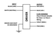
Input and output use lead-wires.
