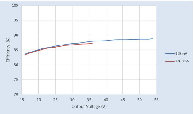
Efficiency Vs. Output Voltage at 277Vac
