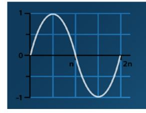
All of the Bodine inverters feature an LED-friendly sinusoidal (sine) waveform rather than square waveform output. Sinusoidal waveform is characterized by very low harmonic distortion and by clean power similar to that produced by utilitysupplied electricity.
