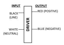
Input and output use lead wires.
