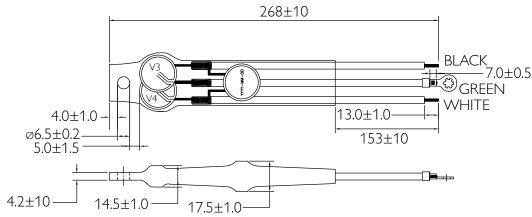
**Caution:** The SP1 surge protection device can have a non-passive failure mode at the end of life, so this device must be always installed inside a fire-resistant enclosure.
