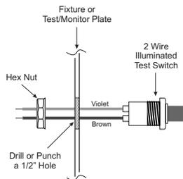
**Note:** The BSL36 Cold-Pak can also be supplied with an IP67 rated test switch intended for mounting on the fixture surface.
