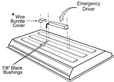
If the application requires the product to be mounted on top of the luminaire please use wire bundle cover kit (RMC-60). Please note, the RMC-60 kit contains enough parts to install two products.
