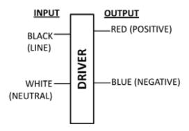
Input and output use lead wires.
