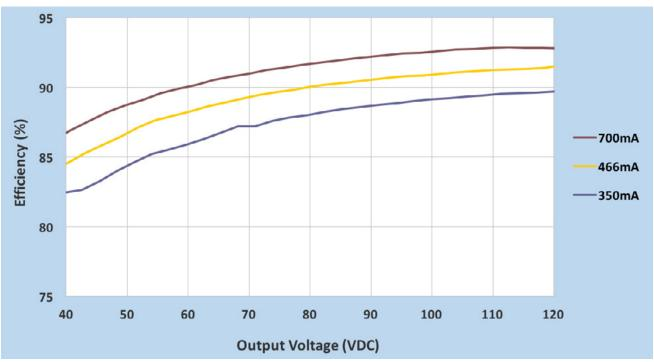
Efficiency Vs. Output Voltage @ 277VAC
