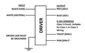
Input lead wires are 18AWG 105C/600V stranded copper with flag terminals per UL1452.
