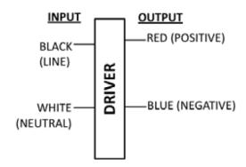
Input and output use lead wires.
