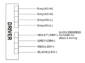
Input and output use lead- wires.
