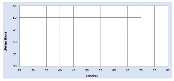
**Performance Characteristics** Based on measurements on a typical sample at 70°C case. The accuracy of the measurements is within the tolerance of the measurement instruments.
