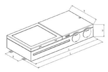
Typical LED forward voltage 36V, over voltage protection threshold >45V.
