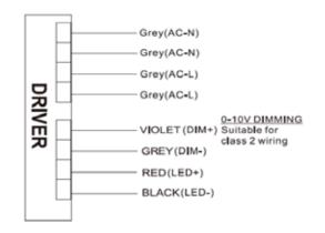
Input and output use lead- wires.
