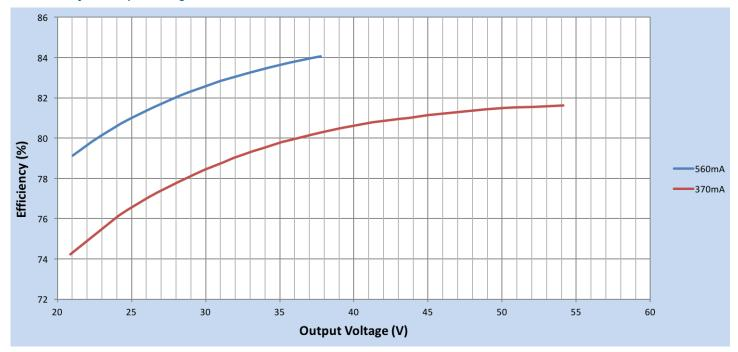
Efficiency Vs. Output Voltage
