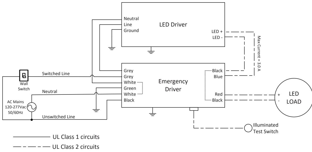
**NOTE:** For short-term testing of the emergency function, the battery must be charged for at least one hour. The emergency driver must be charged for at least 24 hours before conducting a long-term test.
