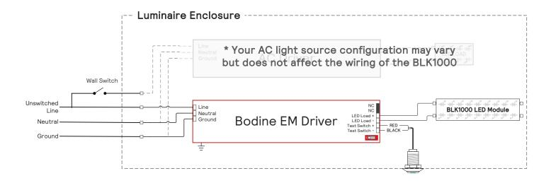
For illustration purposes only. Refer to product installation instructions for actual wiring diagram and proper connection points.
